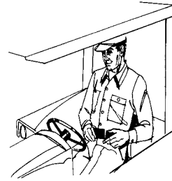
Figure 1. Buckle up if your tractor is equipped with a rollover protective structure.
