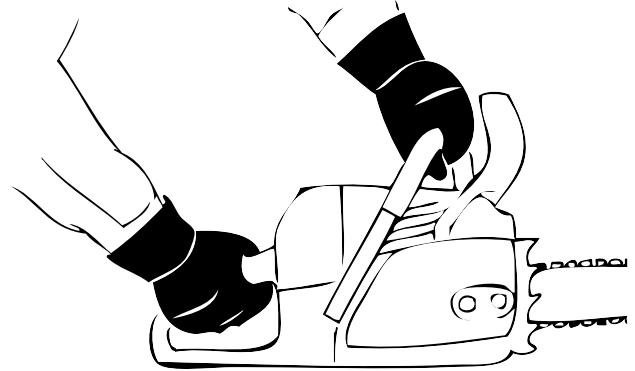
Figure 3. Always maintain a firm grip on the saw with both hands, the left in the front and the right in the back.
