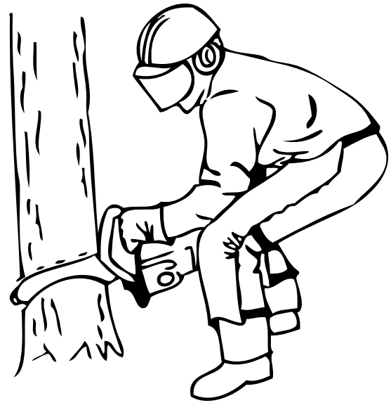
Figure 1. When operating a chain saw, always wear personal protective equipment, including a hard hat, eye and ear protection, gloves and boots.
